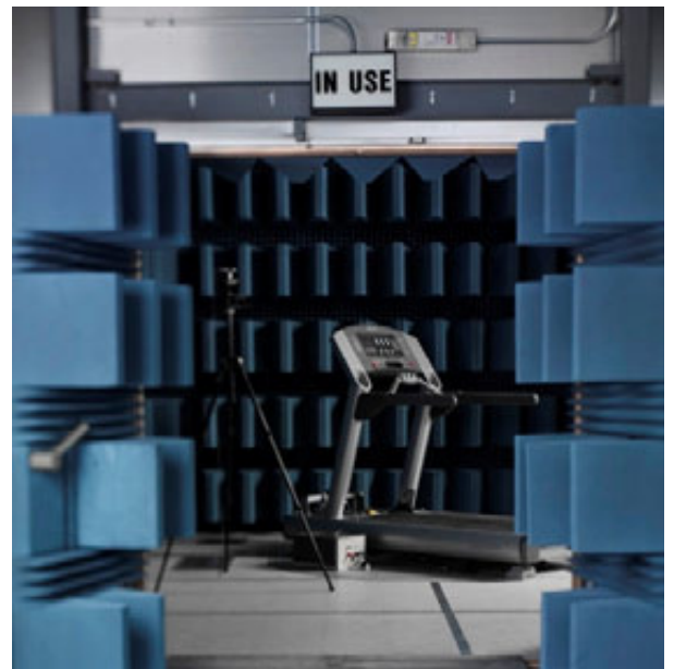
Sound-testing a treadmill
